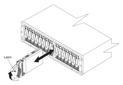
Figure 23. Replacing an E-DDM
